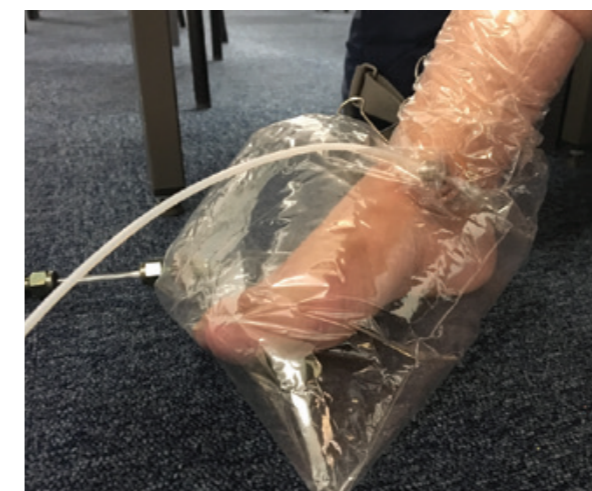
Air entrainment captures the volatile odour compounds released from the skin
