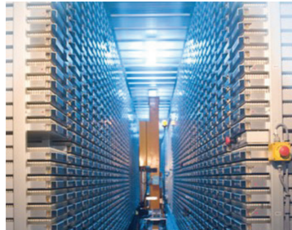
To be able to screen almost 2 million chemical compounds in a short space of time, a highly efficient and automated high throughput screening system such as this is required. Image provided by GSK.
