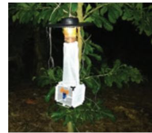
Modified CDC light trap with a sugar-and-dye-soaked FTA card inside a mosquito cage was used in Guinea.
