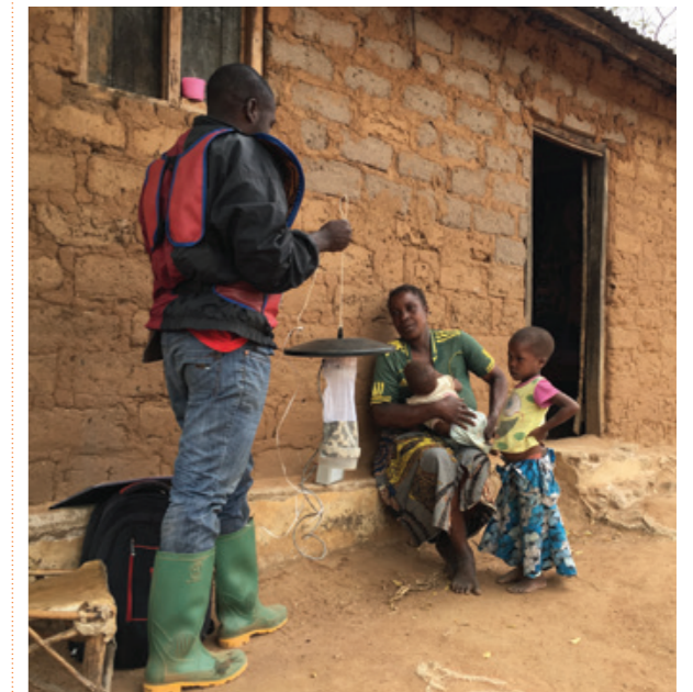
Demonstration of the mosquito trap (CDC light trap) by PAMVERC field assistant during consent procedure, Misungwi, Tanzania
